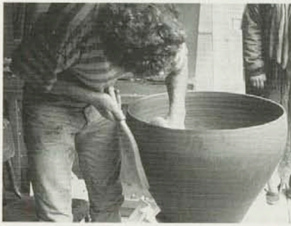
When firm, the rim of the bowl is curved in by beating with a paddle and anvil.
