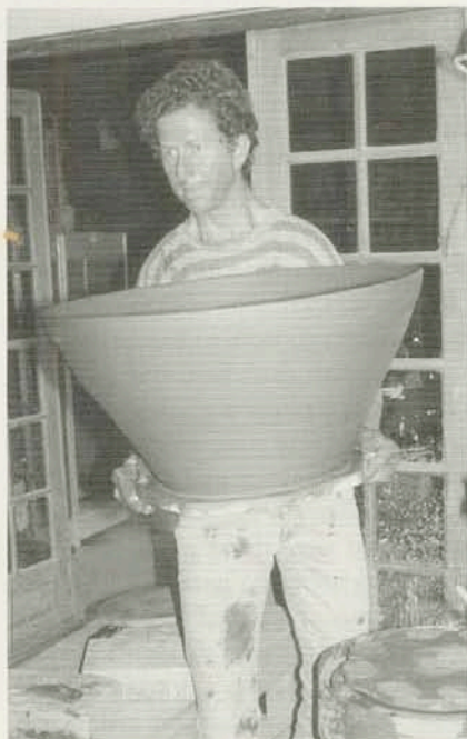
When he is satisfied with its shape, the 26-inch-diameter bowl is removed from the wheel and set aside to dry.
