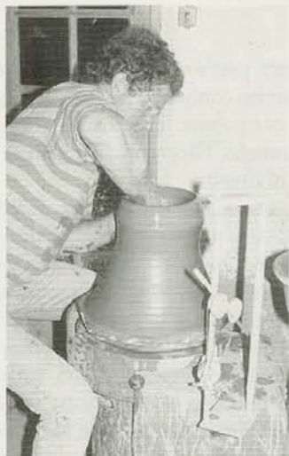
To throw a large planter, Bayer begins by beating 30 pounds of clay into a mound, then centers, opens and pulls.
