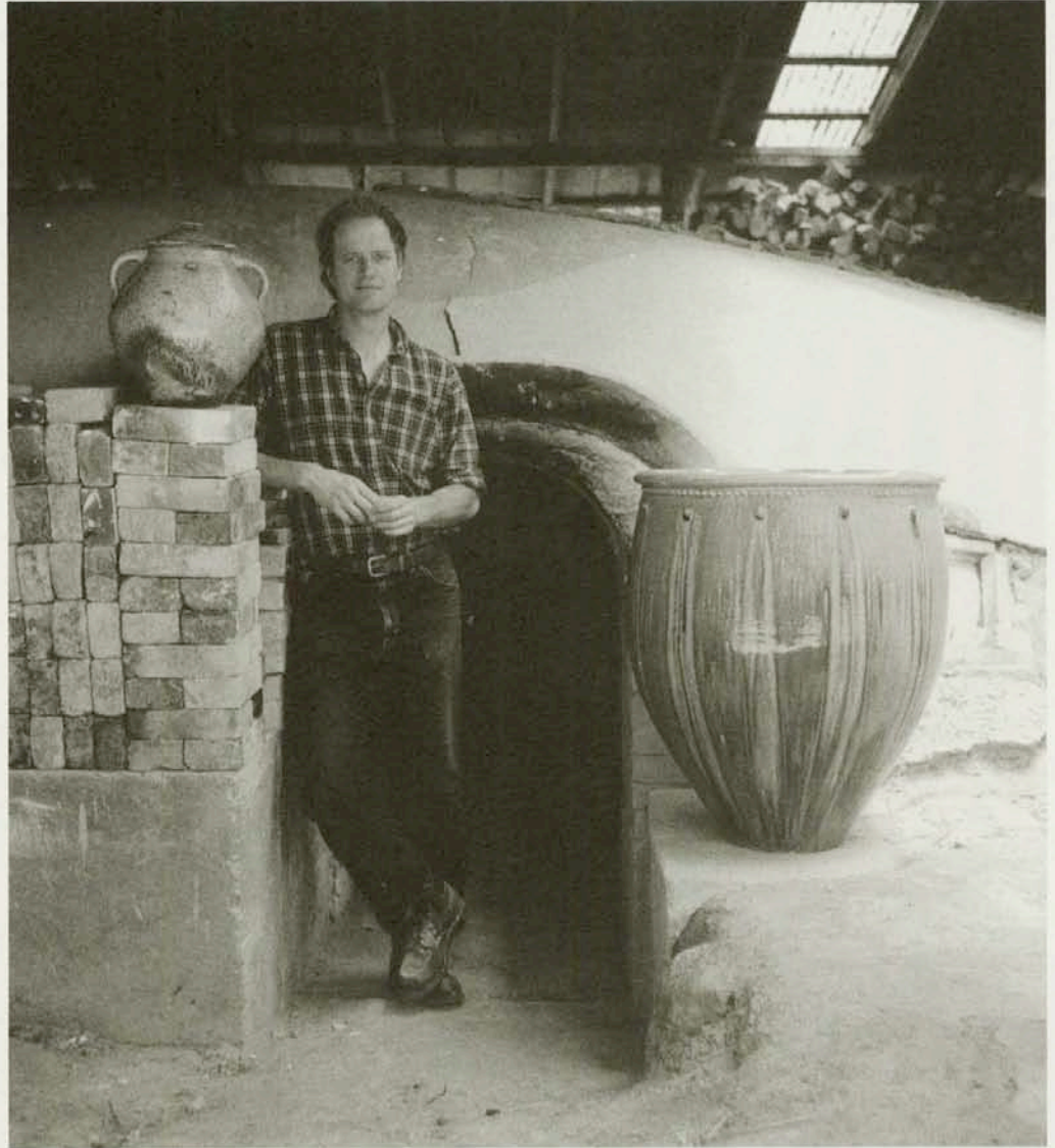
Hewitt at the entrance to his groundhog kiln which can hold up to 1200 pieces of pottery and is fired only three times a year.
